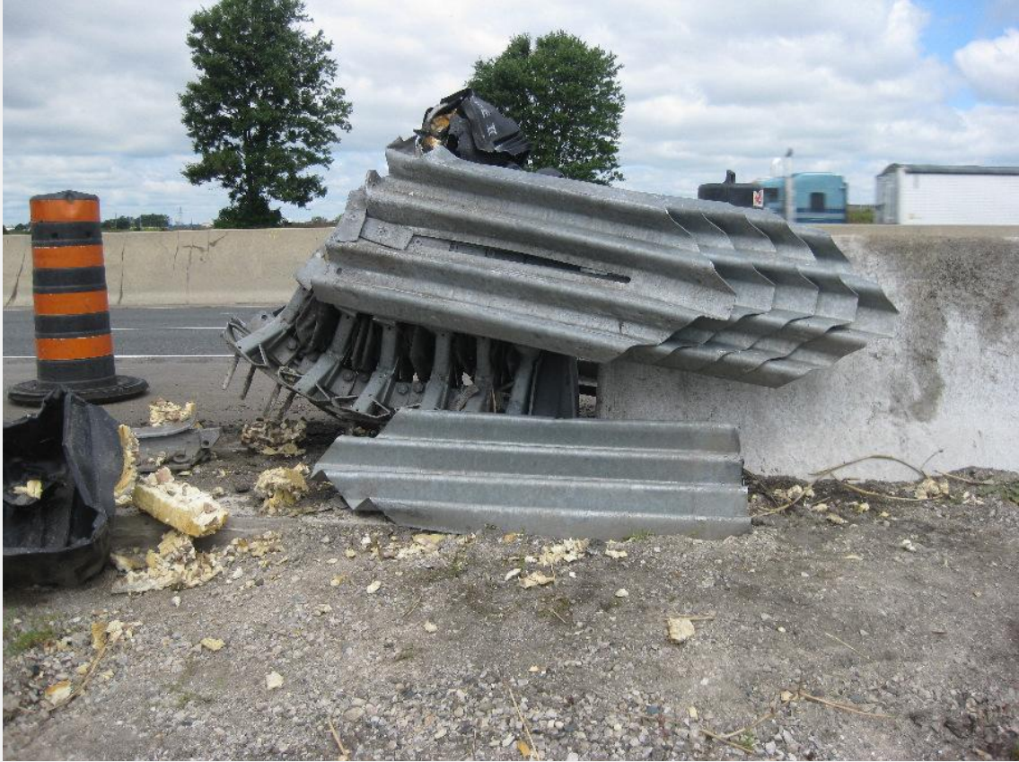
View of the barrier that was fully-compressed by the bus impact.
